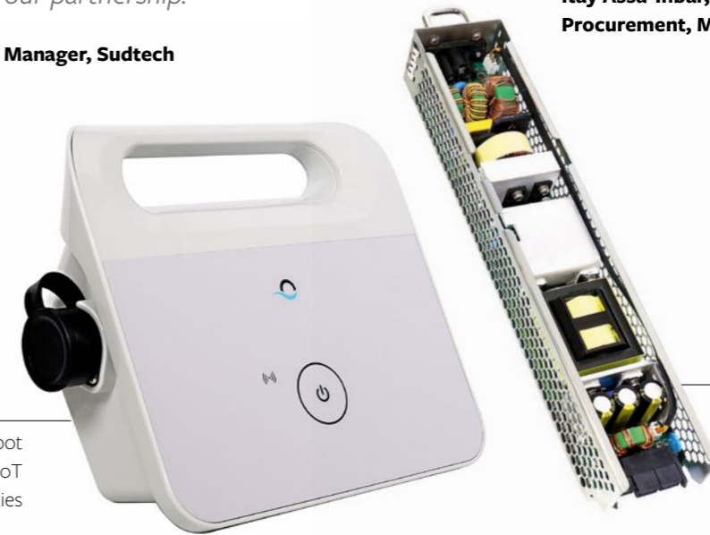
200G high capacity optical transponder power supply with hot-swapping capabilities.
