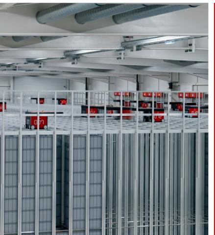
AutoStore is a pioneer and global leader in cubic storage automation. The AutoStore System consists of an aluminum Grid, Robots, Bins, Ports and a Controller. Robots ride on rails along the top of the Grid, retrieving Bins as needed. Using the Router software platform, the Controller constantly adjusts the location and path of Robots in real time.
